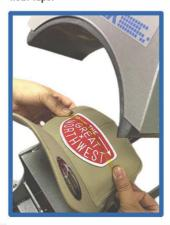
Step 3: With teflon paper on top of emblem, apply heat to hat.
